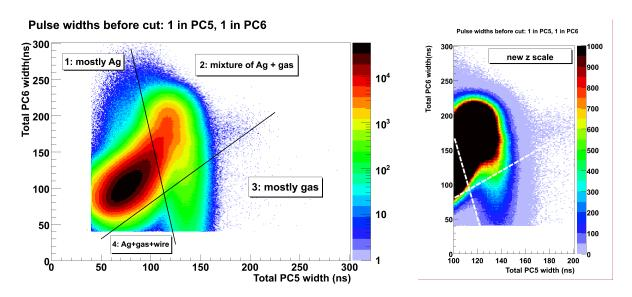
The nearly-vertical cut line runs parallel with the gas band. The gas band has a tail that leaks over this cut line – this is more obvious in the right hand figure, where the scale is changed. We need to estimate how much of the gas band leaks across the zone 1 / 2 boundary to estimate the systematic uncertainty for the psPACT. Specifically, this systematic is "how much gas contamination is left after the psPACT cut".
