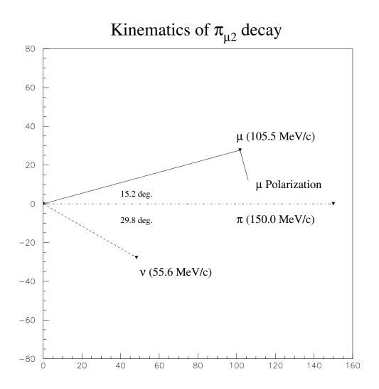
Figure 1: The kinematics for a pion momentum = 150 MeV/c and the muon emitted at the maximum angle. The muon is transversely polarized. Note the direction of the neutrino momentum.
