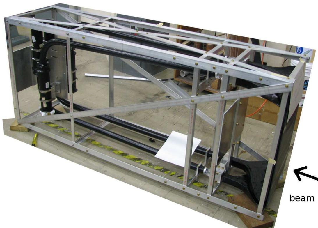
Figure 3.22: Downstream trigger: photograph of completed frame, lightguides, photomultiplier tubes and scintillators.
