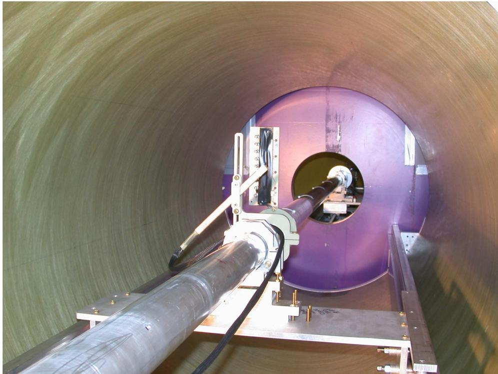
Figure 3.15: A photograph of the field mapper, taken from inside the solenoid. The bore of the magnet has 1 m diameter.
