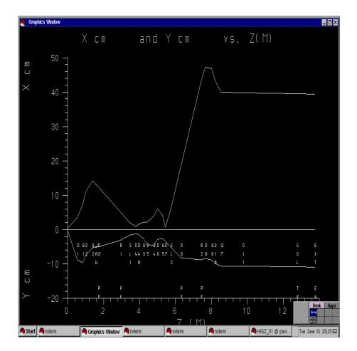
Focusing Effect of the Solenoid, Quads left unchanged
