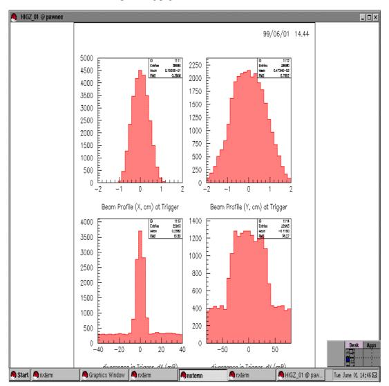
So... Can we figure out where to "find" the good rays? The following obtained by cutting on the previous distribution. Good rays are those which hit a 2cm by 2cm "trigger" (or sweet spot) at the axis of the solenoid, and which have a divergence of less than 10 mR.
