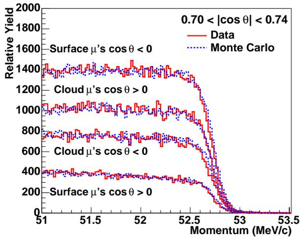
Figure 14: (above) Measured positron momentum spectra (solid lines) near the end point are compared to Monte Carlo simulations (dotted lines). The curves show surface muon set B for  $-0.74 < \cos \theta < -0.70$ , cloud muons for  $+0.70 < \cos \theta < +0.74$ , cloud muons for  $-0.74 < \cos \theta < -0.70$ , and surface muon set B for  $+0.70 < \cos \theta < +0.74$ .
