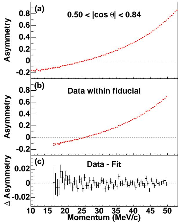
Figure 17: (a) The observed muon decay asymmetry from set B for all events within  $0.50 < |\cos \theta| < 0.84$ . (b) The same quantity for those events that fall within the fiducial region. (c) The difference between the data in panel (b) and the best fit MC spectrum.
