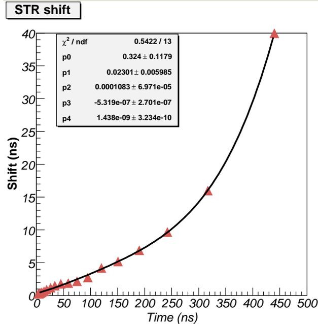
Figure 20: Preliminary comparison of STRs obtained from Garfield simulation to STRs from straight line fits to data.
