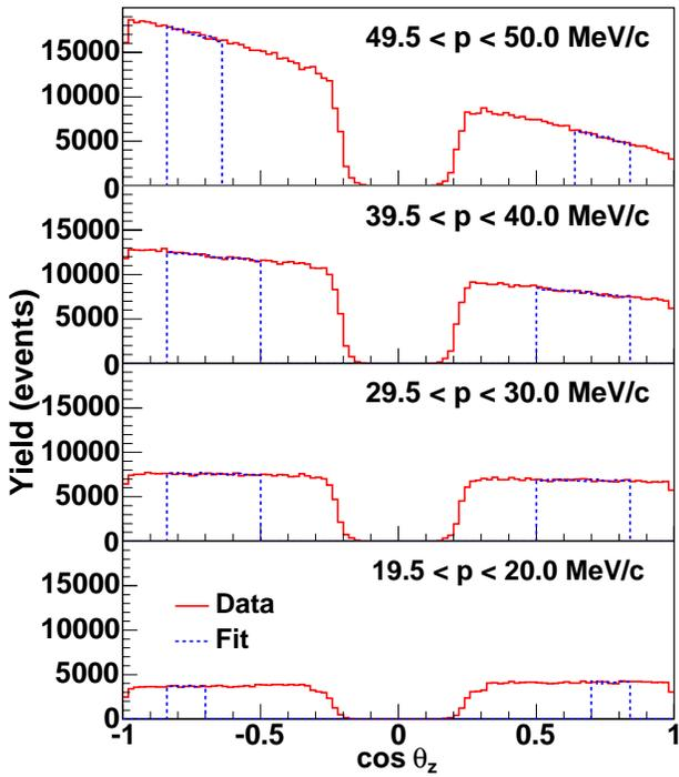
Figure 16: Decay positron angular distributions from set B (solid curves) and the corresponding best fit distributions within the fiducial region (dashed curves) for selected momentum bins.
