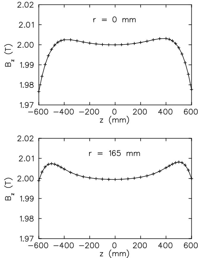
Figure 3: Maps of axial magnetic field, showing  $B_z$  vs.  $z$  for  $x = y = 0$  (upper) and  $r = 165$  mm (lower).
