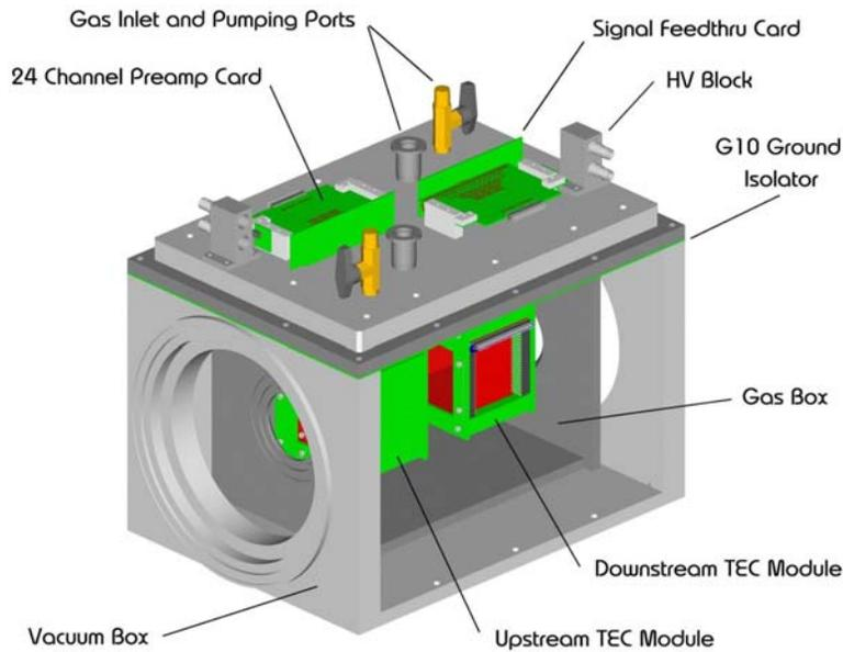
Figure 4: The TEC, showing two modules which measure the position and angle of beam particles, one in  $x$  and one in  $y$ .
