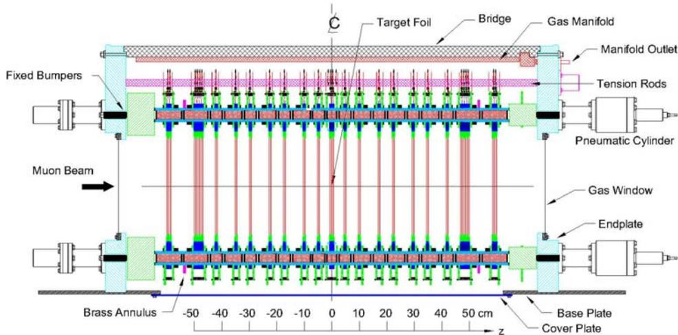
Figure 2: Side view of the symmetric *TWIST* detector stack, showing 19 modules at precise locations along the beam axis.
