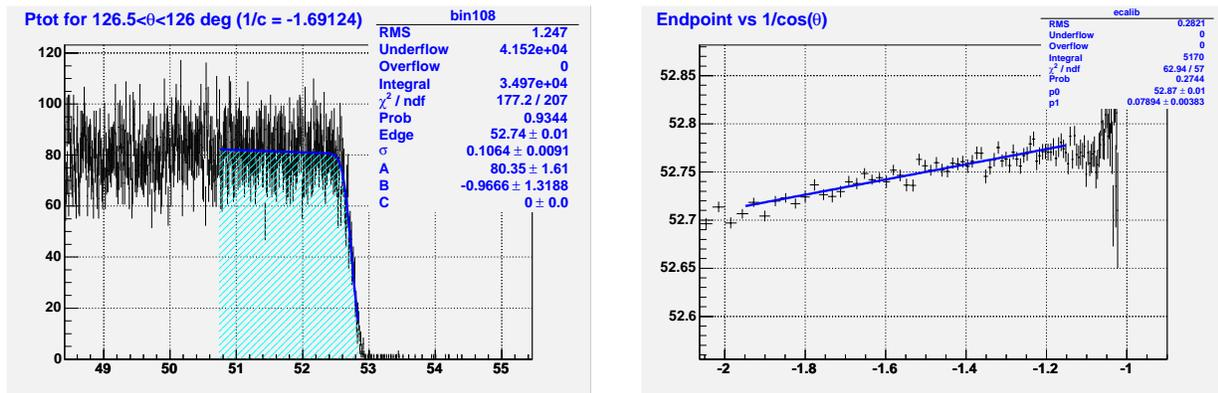
Figure 8: Left panel: Fit to the endpoint. Note that this figure is reproduced from an earlier version of the procedure, which used a different momentum range. Right panel: Angular dependence of the endpoints.
