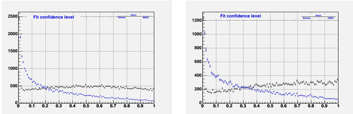
Figure 6: Confidence levels for wire-centre fits to helical tracks for data (left) and simulation (right). The flatter curves are for the fits including kinks.
