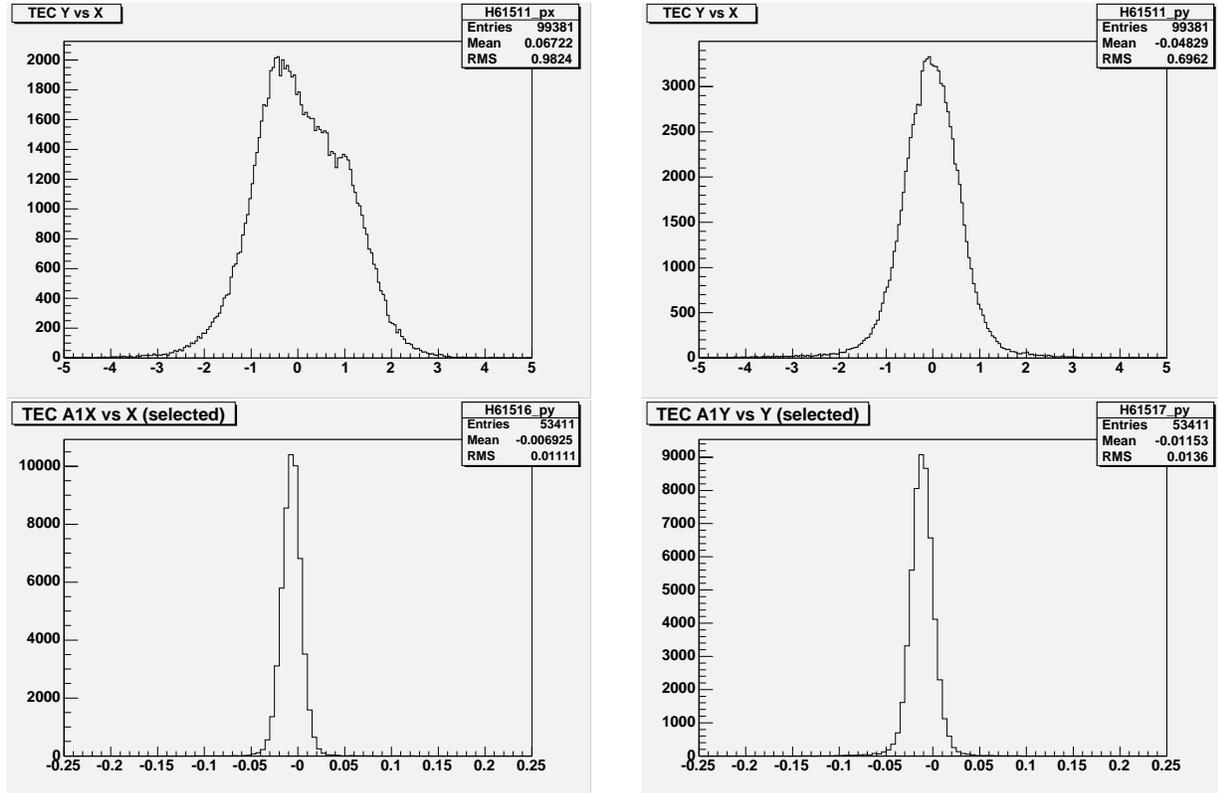
Figure 5: Projections of two-dimensional plots of a surface muon beam produced by a Be production target in a stainless steel water cooling jacket. Plotted are profiles in the  $x$  and  $y$  directions (top), and corresponding distributions of the slopes of individual muon tracks (bottom).
