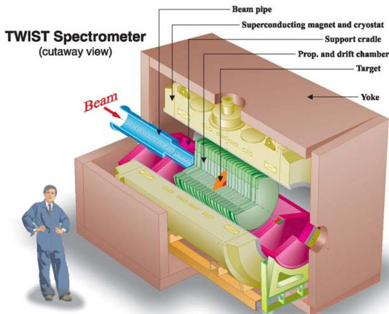
Figure 1: Conceptual drawing of the *TWIST* spectrometer. It shows the superconducting solenoid within the steel yoke, with the drift chambers and proportional chambers symmetrically placed about the central target.
