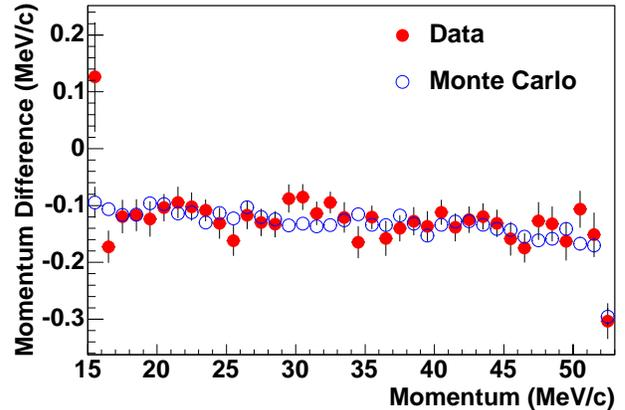
Figure 13: Average energy loss of decay positrons through the target and detector materials as a function of momentum for data (closed circles) and Monte Carlo (open circles), measured as described in the text.
