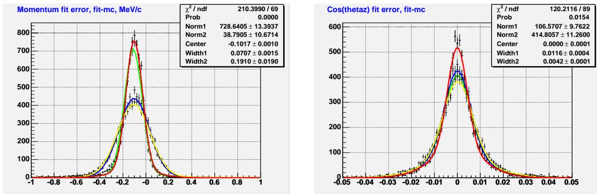
Figure 7: Momentum and angular resolution obtained from various tracking methods. Curves are : drift fit with kinks(red), drift fit no kinks (green), wire centre fit with kinks (blue), wire centre fit no kinks (yellow).
