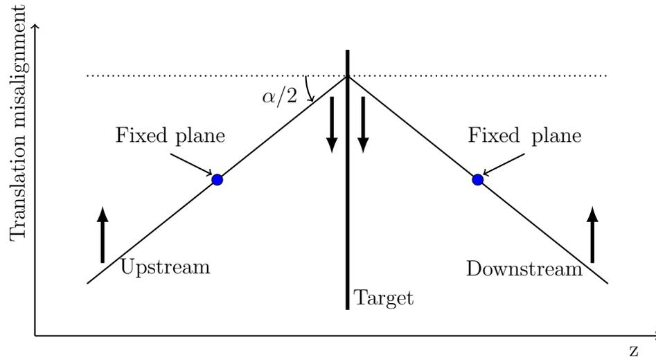
Figure D.2: The kink at the target creates a dependency of the translation misalignment measured with respect to  $z$ . The correction of this effect uses the mean of the kink at the target  $\alpha$  at each iteration. The fixed planes (planes 14 and 31) are used as anchor points for this correction.
