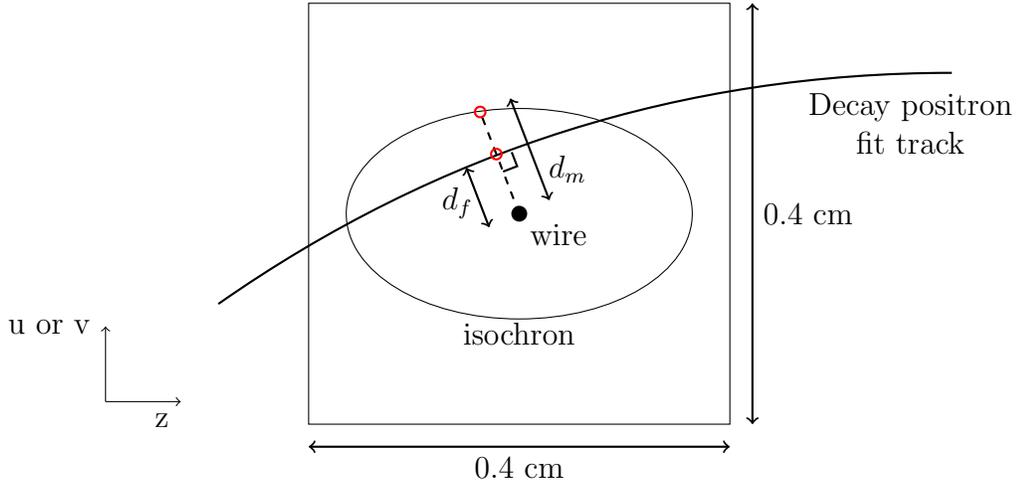
Figure 3.8: Calculation of the drift distances  $d_f$  and  $d_m$  for the  $\chi^2$ . The tangent to the positron track is used in the context of the closest distance of approach. Only the isochron of the measured drift time is drawn here. The difference  $|d_m - d_f|$  is the residual for the hit.
