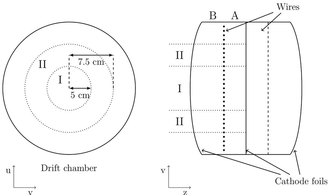
Figure 6.1: The differential pressure between the inside and the outside of a drift chambers module leads to a bulge of the outer cathode foil. In order to compare the bulge between different chambers, the average drift time on the side A of the wires is used as a reference. The foil bulge is given by a difference in average drift times:  $\Delta T = (T_{IA} - T_{IB}) - (T_{IIA} - T_{IIB})$ .
