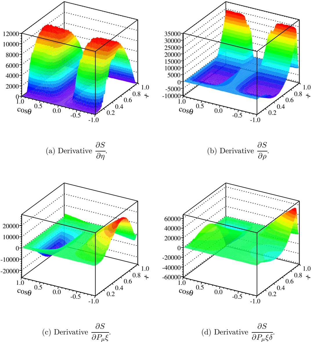
Figure 3.9: The derivative spectra describe the contribution of the decay parameters to the shape of the momentum-angle spectrum. The reduced positron energy  $x = E_e/W_{e\mu}$  is used here instead of the momentum. These spectra include the detector response.
