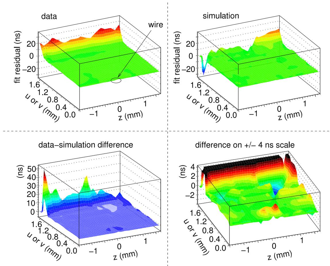
Figure 7.5: The time residuals (Tres) are shown for only half of the drift cell in a DC because the STRs are reflected about  $uv = 0$ . The differences between the 44 data STRs (one per plane) and the global MC STRs (one common to all the planes) define 44  $\Delta$ Tres.
