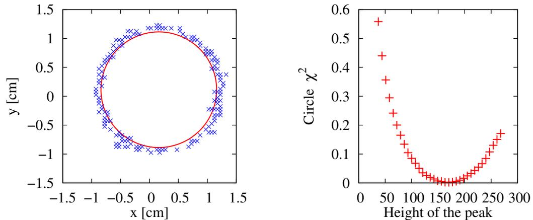
Figure D.5: The cross sections of the track occupancy for a hole are fitted with a circle of constant diameter of 2 cm. The  $\chi^2$  of the circle fits reaches a minimum with respect to the height on the occupancy peak. The circle of minimum  $\chi^2$  is assumed to be best measure the position of the edge of the hole.
