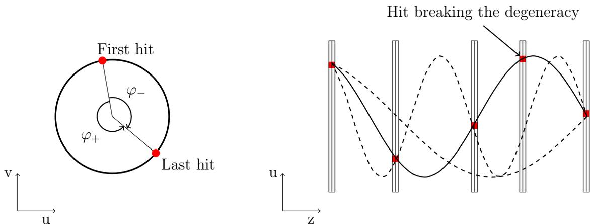
Figure 3.6: Second step in the “first guess” algorithm. The angular difference between the first and the last hit is  $\varphi \pm 2\pi k$  with  $k$  an integer (left diagram). The diagrams are in two dimensions but the algorithm works in three dimensions. This stage of the reconstruction software is vulnerable to degeneracies in the winding numbers. Negative and positive charge tracks are evaluated in parallel ( $\varphi_-$ ,  $\varphi_+$ ).
