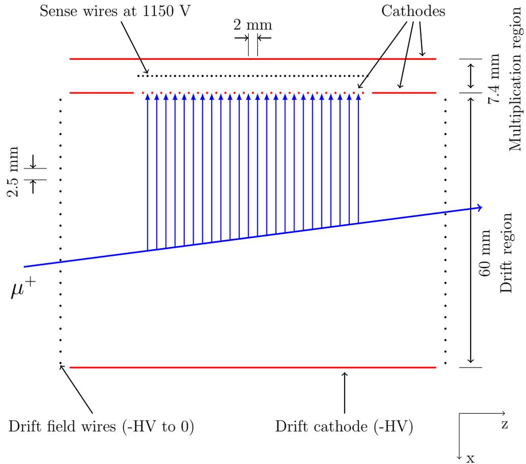
Figure 2.10: Typical event in the  $x$  time expansion chamber. The muon ionizes the DME gas and the free electrons produced drift toward the sense wires because of the drift field created by the drift cathode at a high voltage (HV) of 1000 V. The sense wires are separated by 2 mm with a shield wire in the interval to isolate them from each other.
