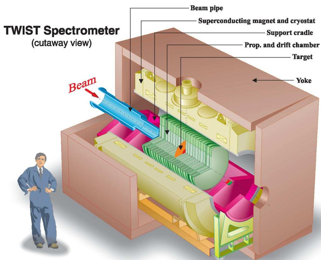
Figure 2.1: The different parts of the TWIST spectrometer are visible in this cutaway view.
