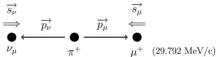
Figure 2.3: The pion decay into a muon and neutrino is the dominant decay mode. In the rest frame, the muon is emitted with a momentum of 29.792 MeV/c and with its spin opposite to its momentum.
