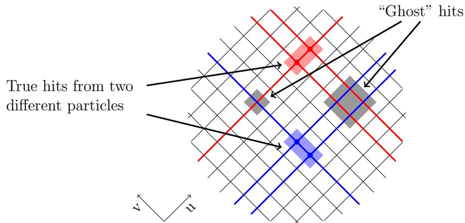
Figure 3.3: Hit clusters formation. Two adjacent wires with a hit are grouped together. The  $u$  and  $v$  hits are associated to have the  $u v$  position of the clusters. In the case of time overlap of two tracks, ghosts clusters appear.
