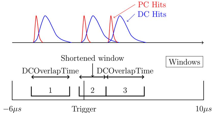
Figure 3.2: This typical event is composed of an early beam positron (window 1), a muon triggering the event (window 2) and a decay positron (window 3). The windows 1 and 3 are of length  $DCOverlapTime$ . The window 2 stops at the beginning of the window 3.
