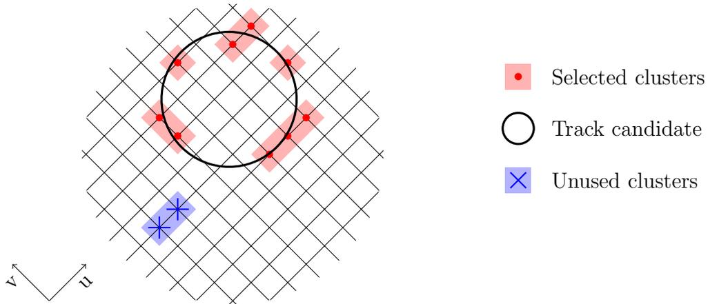
Figure 3.5: The  $u$ - $v$  projection of the hits is fit with various circles from various combinations of three hits. The Chebychev norm is calculated only for the hits or clusters with small enough residuals.
