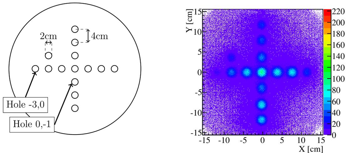
Figure D.4: The collimators installed on the entrances of the yoke contain 14 holes defining a cross plus a hole for the orientation. The holes are labelled using their relative position in  $x$  and  $y$  such that the hole in the center of the cross is the hole 0,0.
