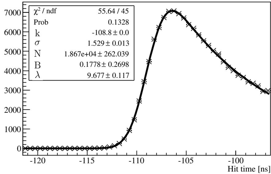
Figure 6.3: The average rising edge is extracted from a fit to the hit times on each wire. The parameter  $k$  defining the position of the step function is the value of the wire time offset for this wire.
