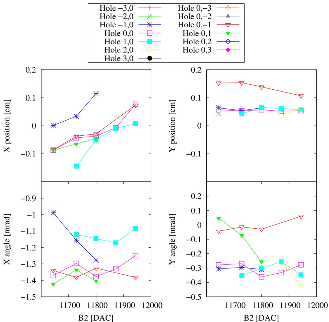
Figure D.6: A change in the B2 DAC value modifies the position and the orientation in  $x$  of the pion beam consequently changing the track occupancy in the holes. For the two extreme B2 DAC values, the beam is centered respectively on the holes -1,0 and 1,0. The measured misalignment between the spectrometer and the yoke is sensitive to the hole occupancy in particular the translational misalignment in  $x$ .
