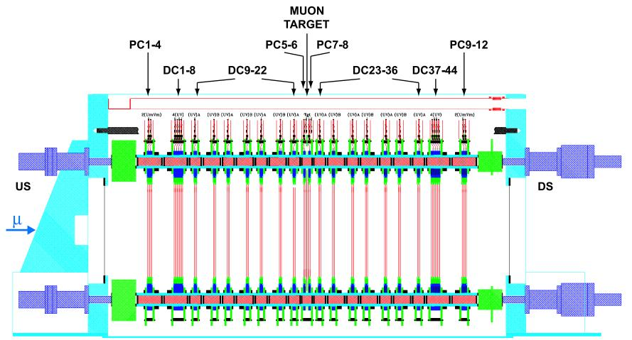
~5000 wires positioned with ~3 micron accuracy.
