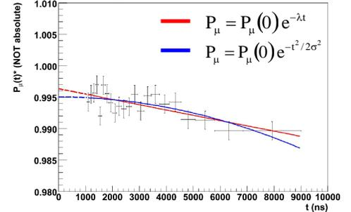
TWIST cannot measure times less than  $\sim 500$ ns, and has not been able to verify the expected exponential form of the depolarisation.
