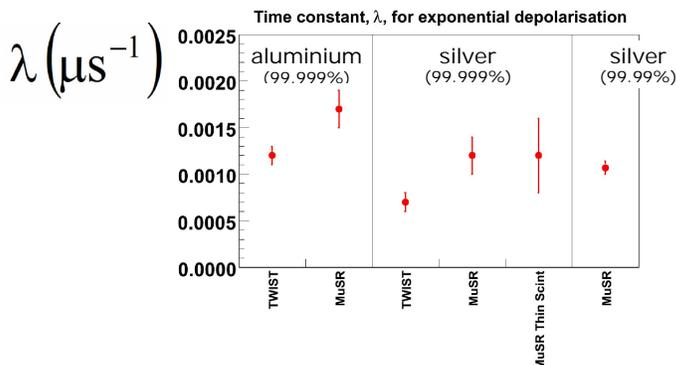
E1111 ( $\mu^+$ SR): no fast depolarisation down to  $\sim 5$ ns
