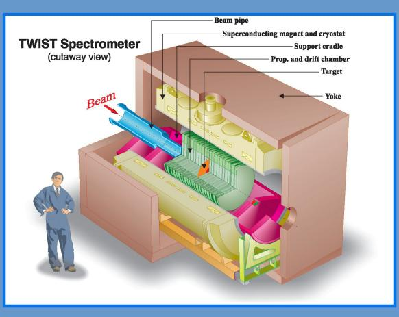
Highly polarized µ<sup>+</sup> stopped in centre of symmetric detector.
