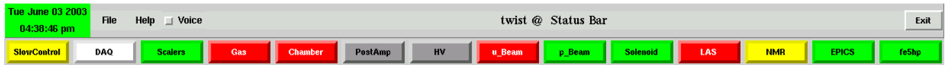
Fig. 7. The Global Status Bar, colors on the buttons indicate the status of the subsystem.: gray=inactive; white=active, not enabled; green=active, enabled; yellow=active, enabled, warning; red=active, enabled, error
