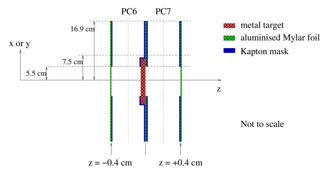
Figure 2.7: The target module is different from the two other PC modules. The stopping target acts as the cathode foil between PC 6 and PC 7.
