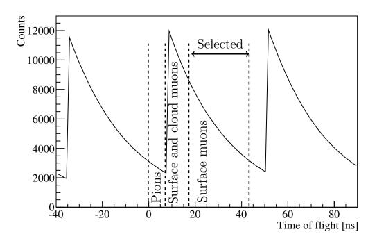
Figure 4.2: Time of flight structure of the beamline M13 at 29.6 MeV/c is periodic due to the cyclotron emitting protons every 43 ns. The main component is the surface muon distribution which is the exponential decay rate of the pion with a time constant of 26 ns. The pions and cloud muons on the other hand are prompt and therefore peaked around their respective time of flight.
