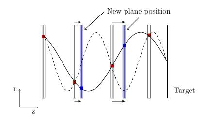
Figure 2.6: Several of the sparse stack DCs were moved prior to this measurement in order to reduce the degeneracies in the track reconstruction such as for this upstream decay. This schematic does not represent the actual geometry of the spectrometer.
