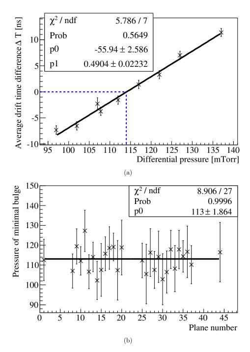
Figure 6.2: The cathode foil is flat if the difference between the average drift times of center and the outside of the chamber is zero . (for example for plane 13 on Fig. (a)). The pressure of minimum bulge is taken from an average for all the planes (Fig. (b)).
