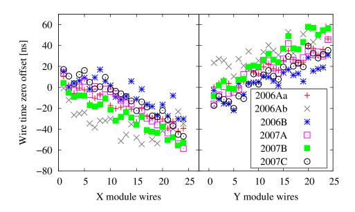
Figure C.4: The main source of the vertical shift of the time offsets is mostly due to the temperature of the DME gas. The difference in slopes is due to different positions of the different sense wire planes from their nominal values.
