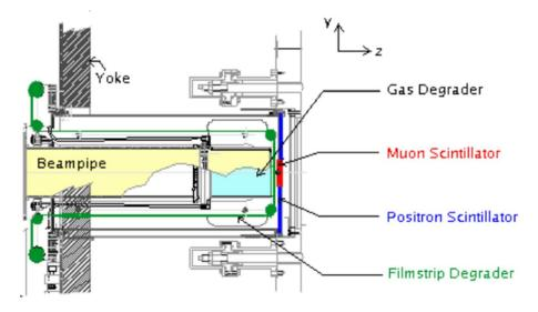
Figure 2.8: The beam package assembly includes the muon counter and the PU scintillator as well as their respective photomultipliers. It also contains the gas degrader which adjusts the stopping distribution of the muons in the spectrometer.
