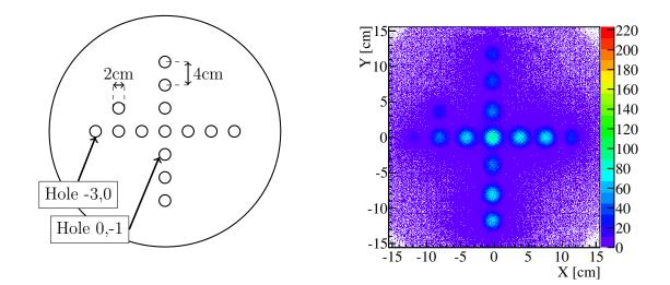
Figure D.4: The collimators installed on the entrances of the yoke contain 14 holes defining a cross plus a hole for the orientation. The holes are labelled using their relative position in x and y such that the hole in the center of the cross is the hole 0,0.
