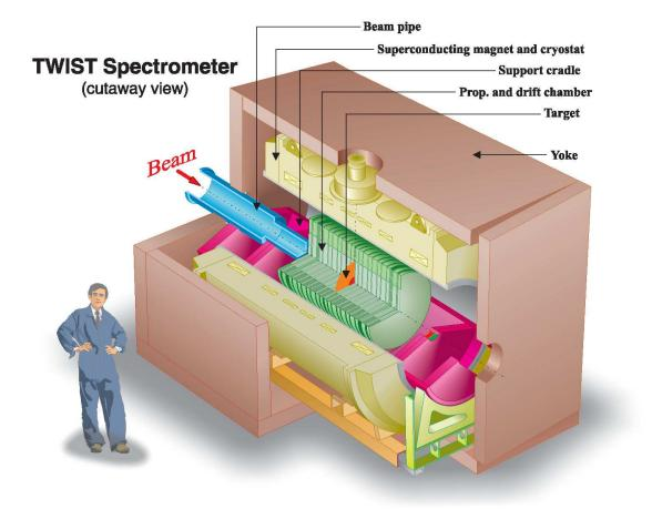
Figure 2.1: The different parts of the TWIST spectrometer are visible in this cutaway view.
