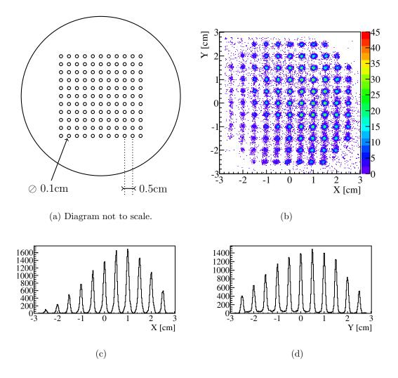
Figure C.2: Diagram of the collimators installed on the TEC gas box in (a). The corresponding profile measured by the TEC is (b). Only the projections on x or y in (c) and (d) are measured by the wires.
