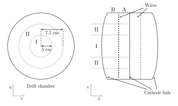
Figure 6.1: The differential pressure between the inside and the outside of a drift chambers module leads to a bulge of the outer cathode foil. In order to compare the bulge between different chambers, the average drift time on the side A of the wires is used as a reference. The foil bulge is given by a difference in average drift times:  $\Delta T = (T_{\rm IA} - T_{\rm IB}) - (T_{\rm IIA} - T_{\rm IIB}).$
