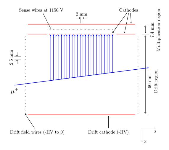
Figure 2.10: Typical event in the x time expansion chamber. The muon ionizes the DME gas and the free electrons produced drift toward the sense wires because of the drift field created by the drift cathode at a high voltage (HV) of 1000 V. The sense wires are separated by 2 mm with a shield wire in the interval to isolate them from each other.
