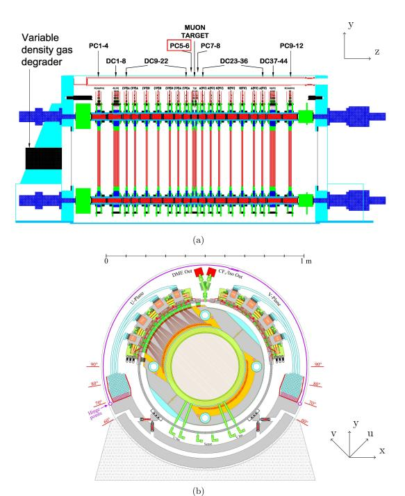
Figure 2.5: The side cross section of the detector (Fig. (a)) shows the 56 planar wire chambers installed symmetrically around the muon stopping target. A system of pneumatic cylinders keep precisely in place the chambers for the duration of the run period. The wires are oriented parallel to the u or v axis (u plane shown on Fig. (b)). The uvz coordinate system is equivalent to the xyz coordinate system rotated by  $45^{\circ}$  around the z axis.
