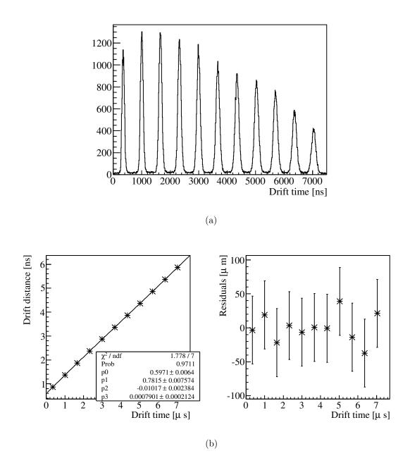
Figure C.8: The eleven drift time peaks are fitted independently in (a) with a Gaussian distribution to obtain the mean. The plot (b) of the drift distance versus the drift time is fitted with a third order polynomial which represents the space time relation for this wire. The error bars on the residuals are the uncertainties on the hole positions on the collimators.
