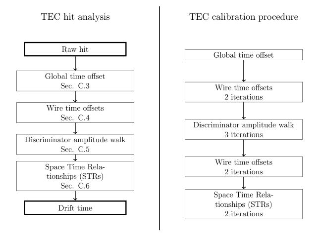
Figure C.1: Four calibrations are applied to a raw hit before obtaining the drift time (on the right). The TEC calibration procedure measures the four calibrations. Most calibrations require few iterations due to the interplay between the track reconstruction and the calibrations. The discriminator amplitude walk correction affects the wire time offsets. For this reason the wire time offsets are calibrated before and after the discriminator amplitude walk correction is measured.
