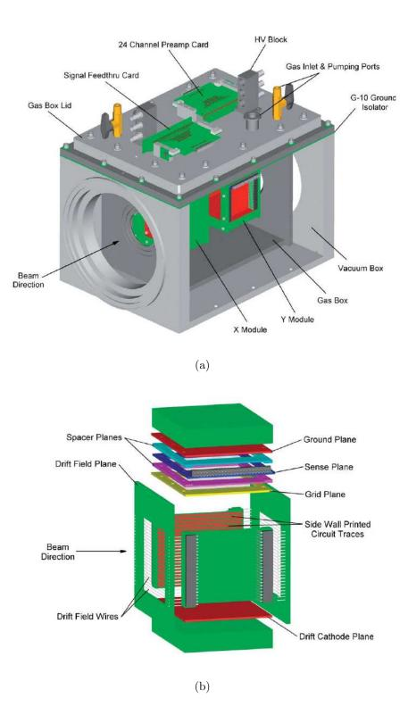
Figure 2.9: Two time expansion chambers are installed the gas box (Fig. (a)). The gas box and the TEC electronics are removed from the vacuum box for nominal data measurement. The vacuum box is a permanent element of the M13 beamline. Both time expansion chambers are identical and measure respectively the x and y directions (Fig. (b)).
